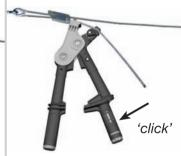
4. When the handle clicks, the desired tension has been reached and the handle will displace.
