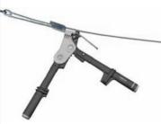
Position the tool mouthpiece against the Gripple, and grip the tail wire with the cam.
