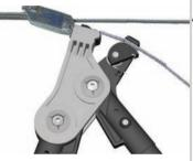
Rotate the dial to tension required. Open the tool handles fully, a sharp pull opens the cam to grip the wire.
