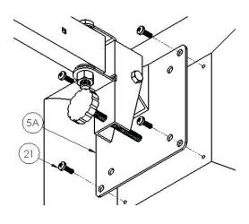
Step 7: Attaching the monitor to the mounting plate
