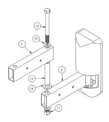
Step 5: Attaching the front force arm to the rear force arm
