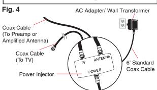
NOTE: This power supply is equipped with a Polyswitch. If there is a short between the preamp and the power supply, it will shut the power supply off until the short is removed.
