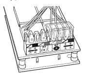
Place the second set of wires into the terminal following the color code.
