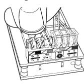
Punch-down the wires then snap the punch-down cap in place.
