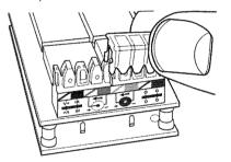
Place the wires into the punch-down slots following the color code shown on the terminal.
